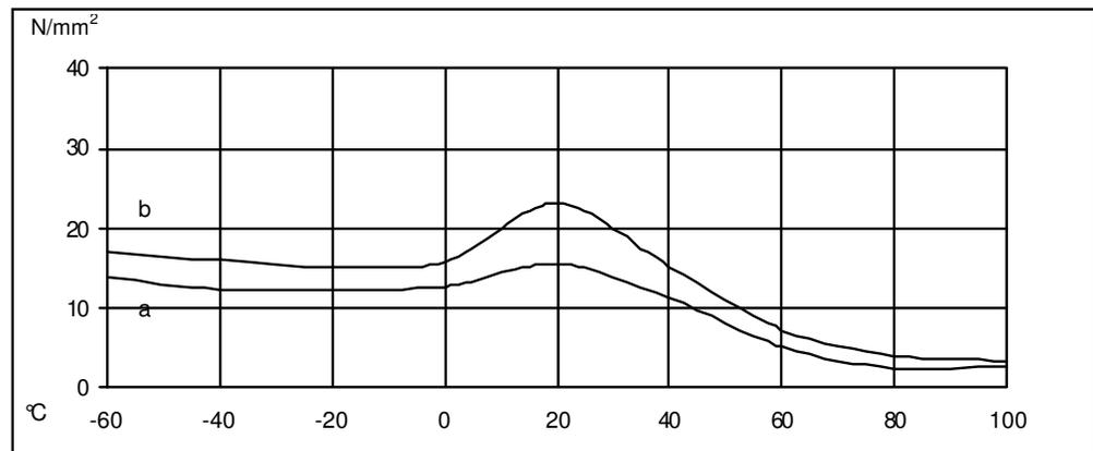
**Roller peel test (ISO 4578) (typical average values)**
