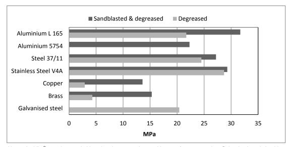
Notes: Araldite<sup>®</sup> 2051 is not suitable to bond copper or brass without surface preparation. Galvanised steel should not be abraded or sandblasted, better results are obtained with only degreasing.
