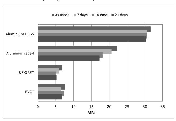
(\*): UP-GRP, PVC, substrate failure
